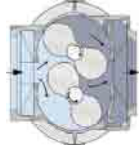
Lower air pocket about to be sealed off at inlet.
