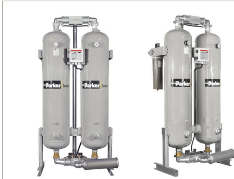
The K-MT 10-95 adsorption dryer series operates a fixed, timed, changeover-cycle between the two dryer vessels. Where the application calls for a unit able to cope with variations in operating pressure and load, the installation of a dew point sensor at the outlet of the dryer is available as an option: In such an operating mode, the changeover-cycle between vessels only takes place when required, and is
